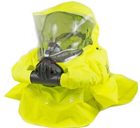
The Semmco HEAD 15 RPE/CSRE Set is a self-contained, short duration oxygen (O<sub>2</sub>) rebreather that provides 15 minutes wearer protection for those working in prisons, detention centres and immigration centres. It enables a safe rescue or working in environments that are affected by smoke, toxic contamination and oxygen deficiency.
